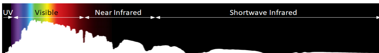
Figure 11 Electro-magnetic & Solar Spectrum 300 – 2500nm
