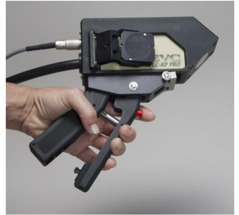
When the LC-RP PRO is used as a Contact Probe, the detachable leaf clip assembly is conveniently parked in the protected recess of the unit. Power is delivered from an i-Series instrument or by an optional battery pack.
