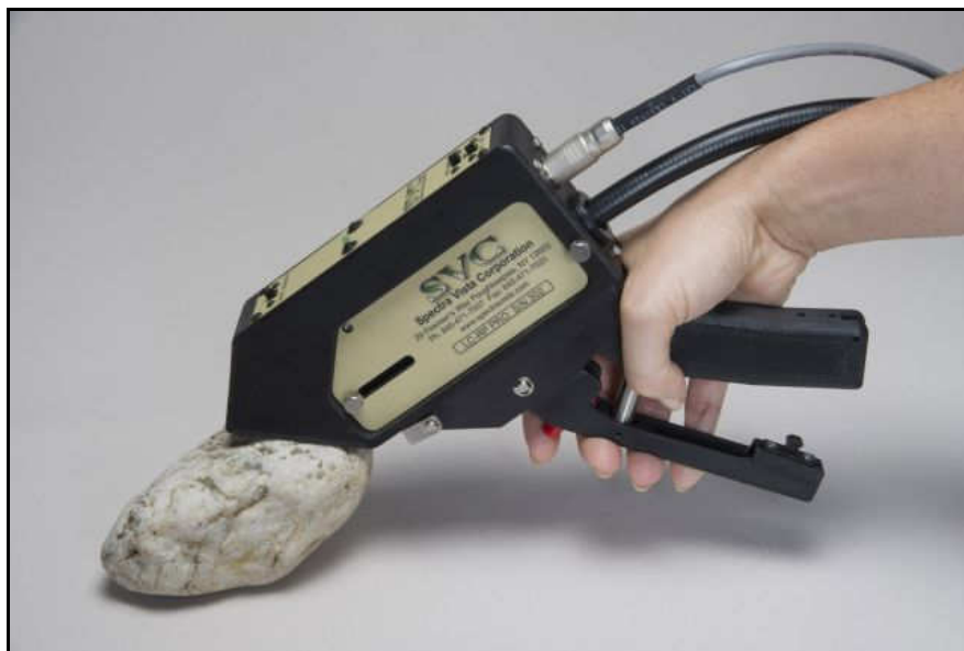
Figure 2 Using the LC-RP PRO in Contact Mode
