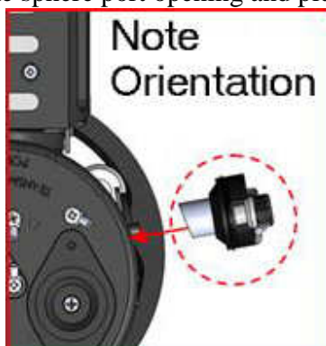
Figure 18: Port plug correct orientation
