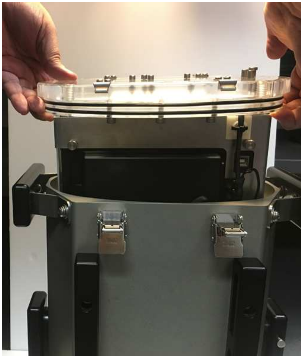
Figure 16 Lowering Rear Panel Assembly Into Enclosure
