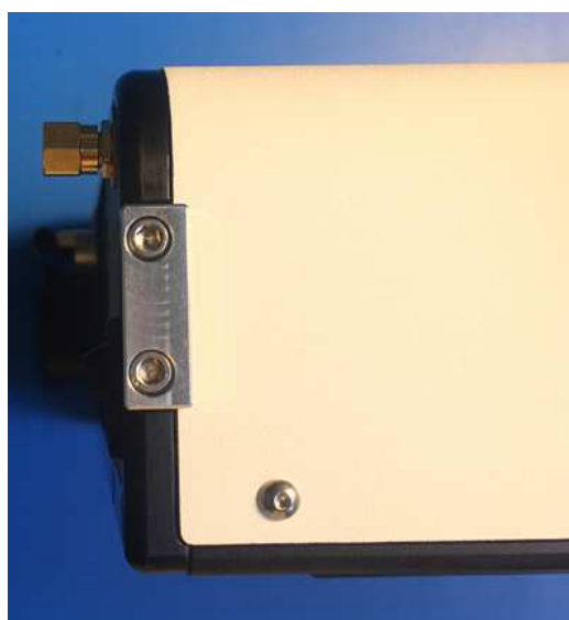
Figure 7 Trim Blocks (Right Side Shown) Installed
