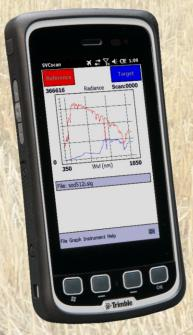
The PDA can withstand drops from 4 ft., accidental immersion, exposure to sand and dust, vibration and extreme temperatures from -30° C to 60° C. The battery provides power for up to 10 hours of operation.
