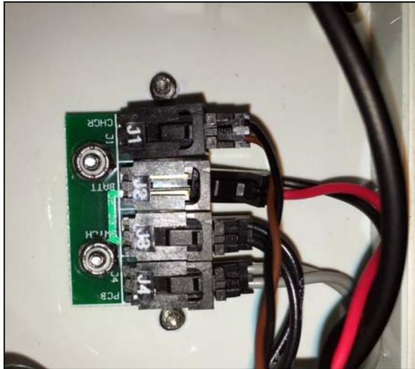
Figure 24 Battery Replacement - Connector J2 "BATT" Partially Removed
