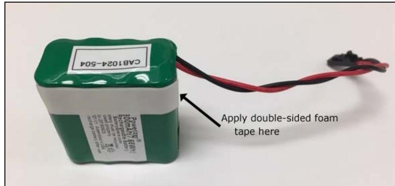
Figure 26 WEDI-4 Battery With Foam Tape Applied
