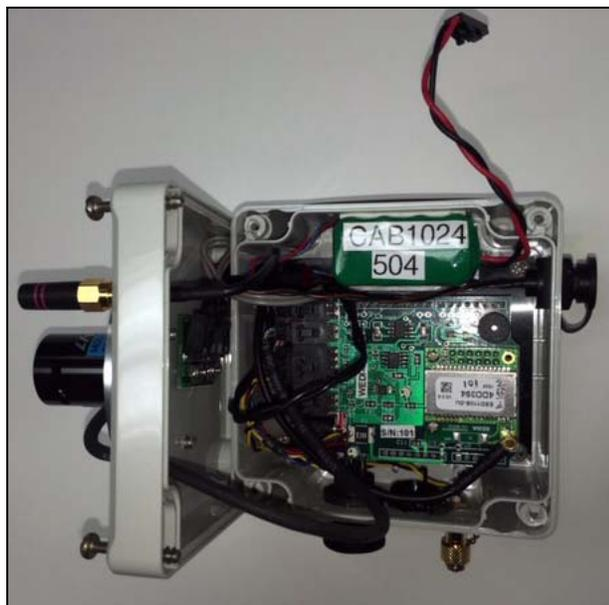
Figure 25 Battery Replacement - Old Battery Prepared For Removal
