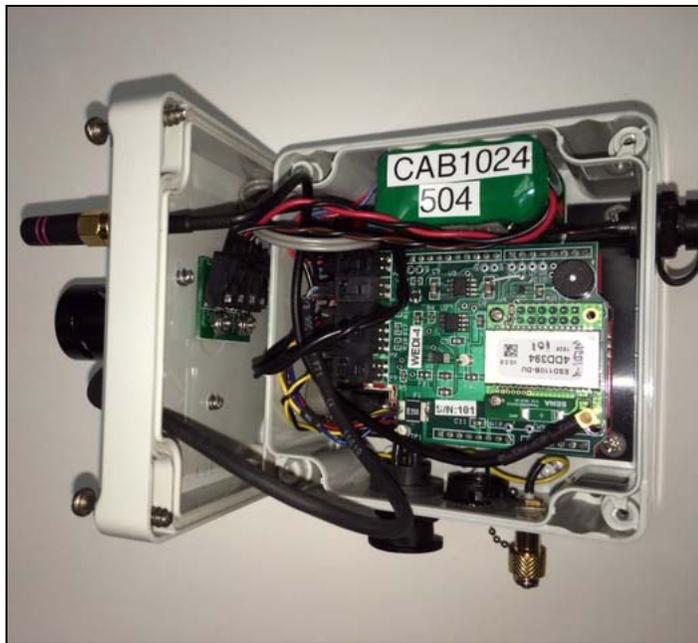
Figure 23 Battery Replacement – Opening The Unit
