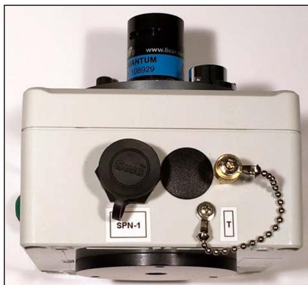
Figure 2 WEDI-4 Side View Showing External Sensor Inputs – Pyranometer (SPN-1), and Thermistor (T)
