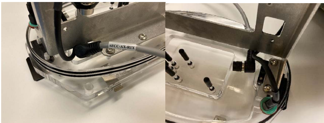
Figure 20 Installing AUX Port Cable Onto The Front Door.
