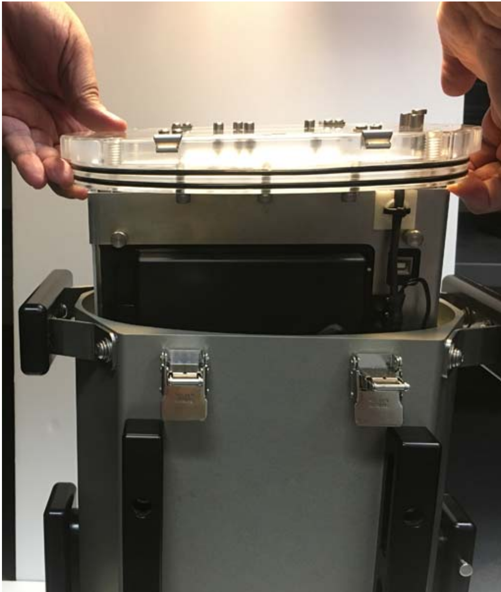
Figure 15 Lowering Rear Panel Assembly Into Enclosure
