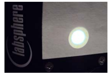
Good beam alignment
