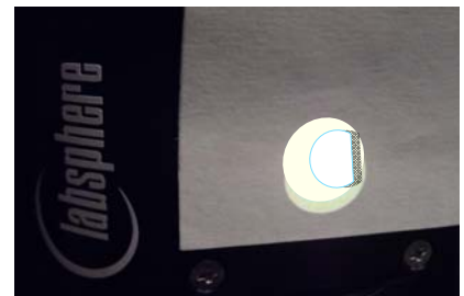
Beam needs alignment (Clipping Entrance Port)
